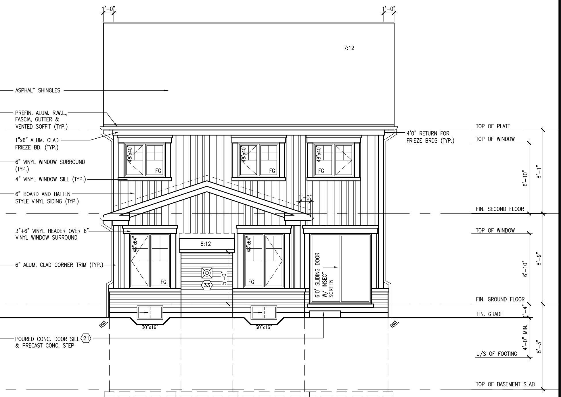
REAR UPGRADE ELEVATION 'B'
