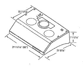
MOUNTING HEIGHTS Minimum height 26" from cooking surface. Hood mounted 60" from floor.
