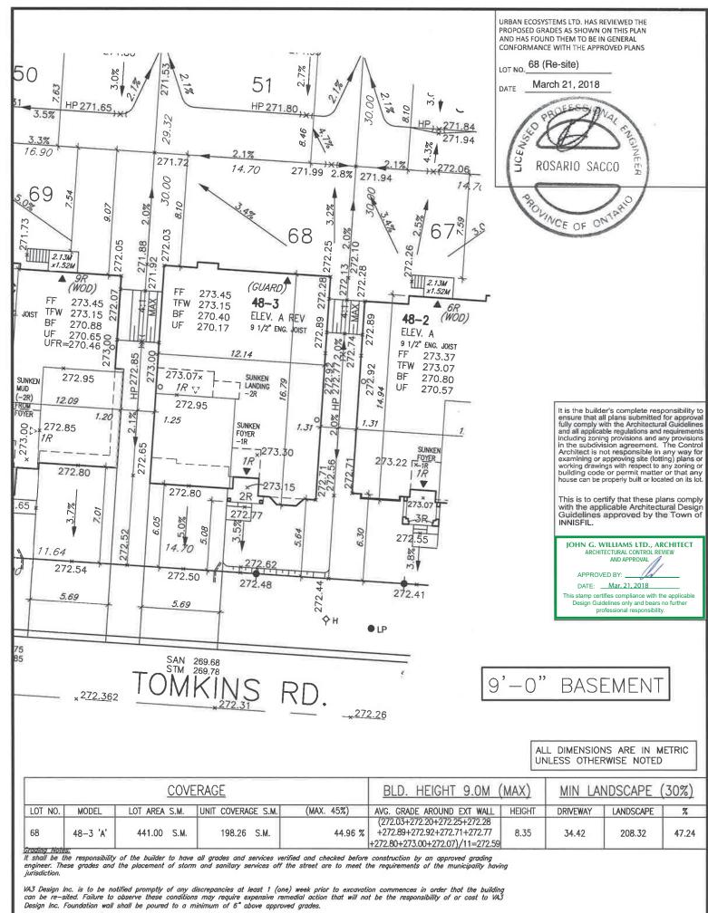
Finished grade lines as indicated on the house prototype are for reference only and do not necessarily depict finish grading conditions of any particular lot.
