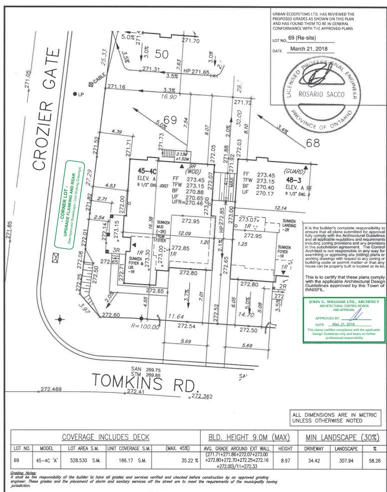
VA3 Design Inc. is to be notified promptly of any discrepancies at least 1 (one) week prior to excavation commences in order that the building can be re-sited. Failure to observe these conditions may require expensive remedial action that will not be the responsibility of or cost to VA3 Design Inc. Foundation wall shall be poured to a minimum of 6" above approved grades.
