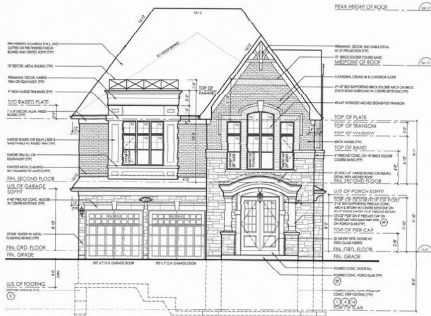
FRONT ELEVATION 'B' UPGRADE
