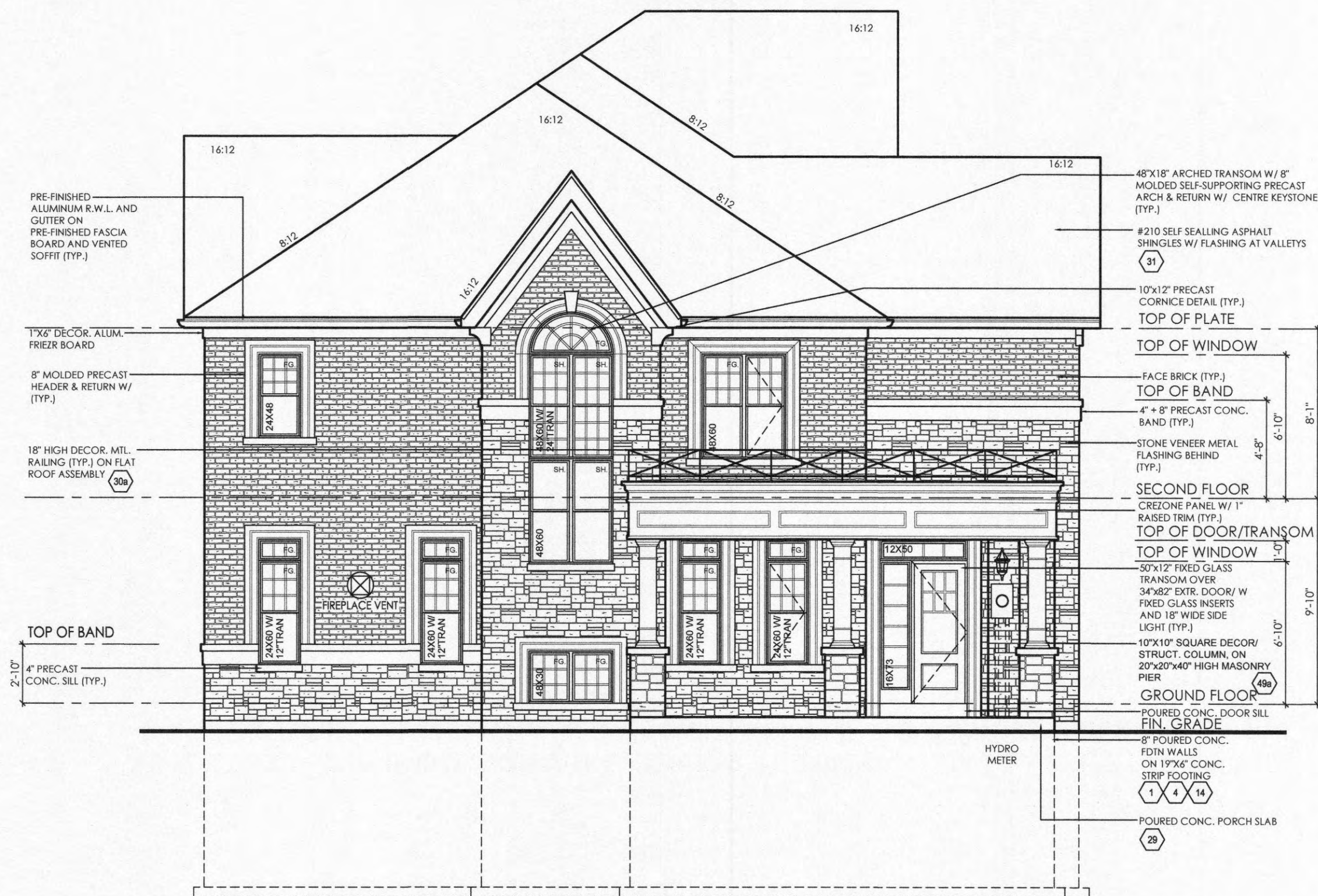
LEFT ELEVATION 'C' CORNER UPGRADE
