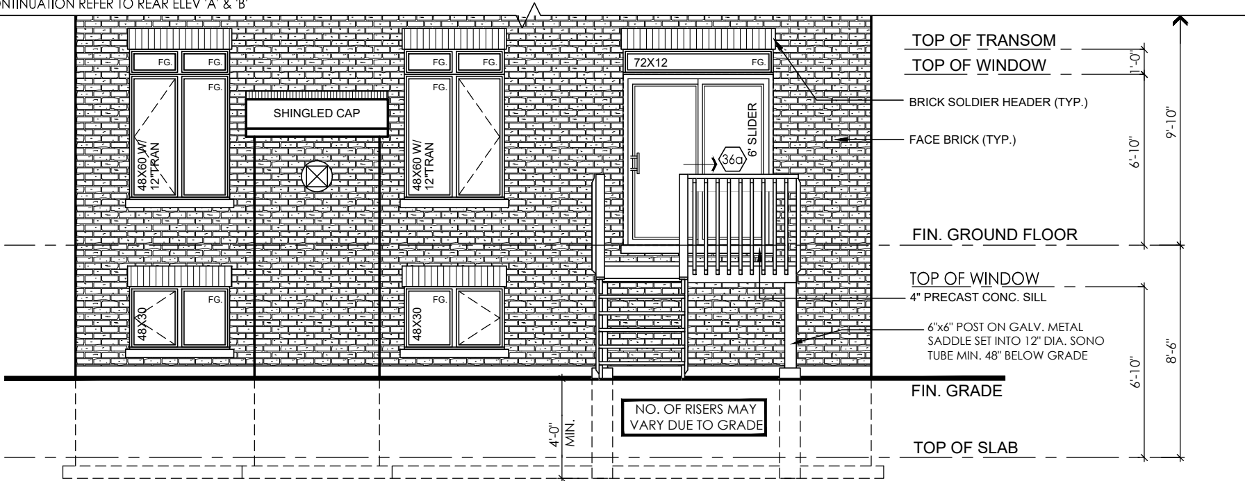
PARTIAL REAR ELEVATION 'A' & 'B' LOB CONDITION
