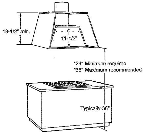
**NOTE:** The exhaust duct on the hood is closer to the rear of the hood. It is important to plan for the alignment to the connection point of the hood.
