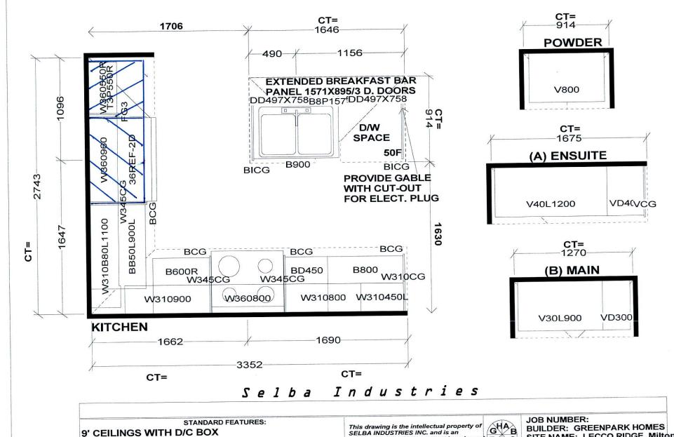
9' CEILINGS WITH D/C BOX 1040MM HIGH UPPER CABINETS DISHWASHER SPACE **DUMMY DOORS ON EXPOSED BACKS** LAMINATE KITCHEN & VANITY COUNTERTOPS SELBA INDUSTRIES INC. and is an original desigh which must not be released FEDC or copied unless applicable fee has been paid or job order placed.
