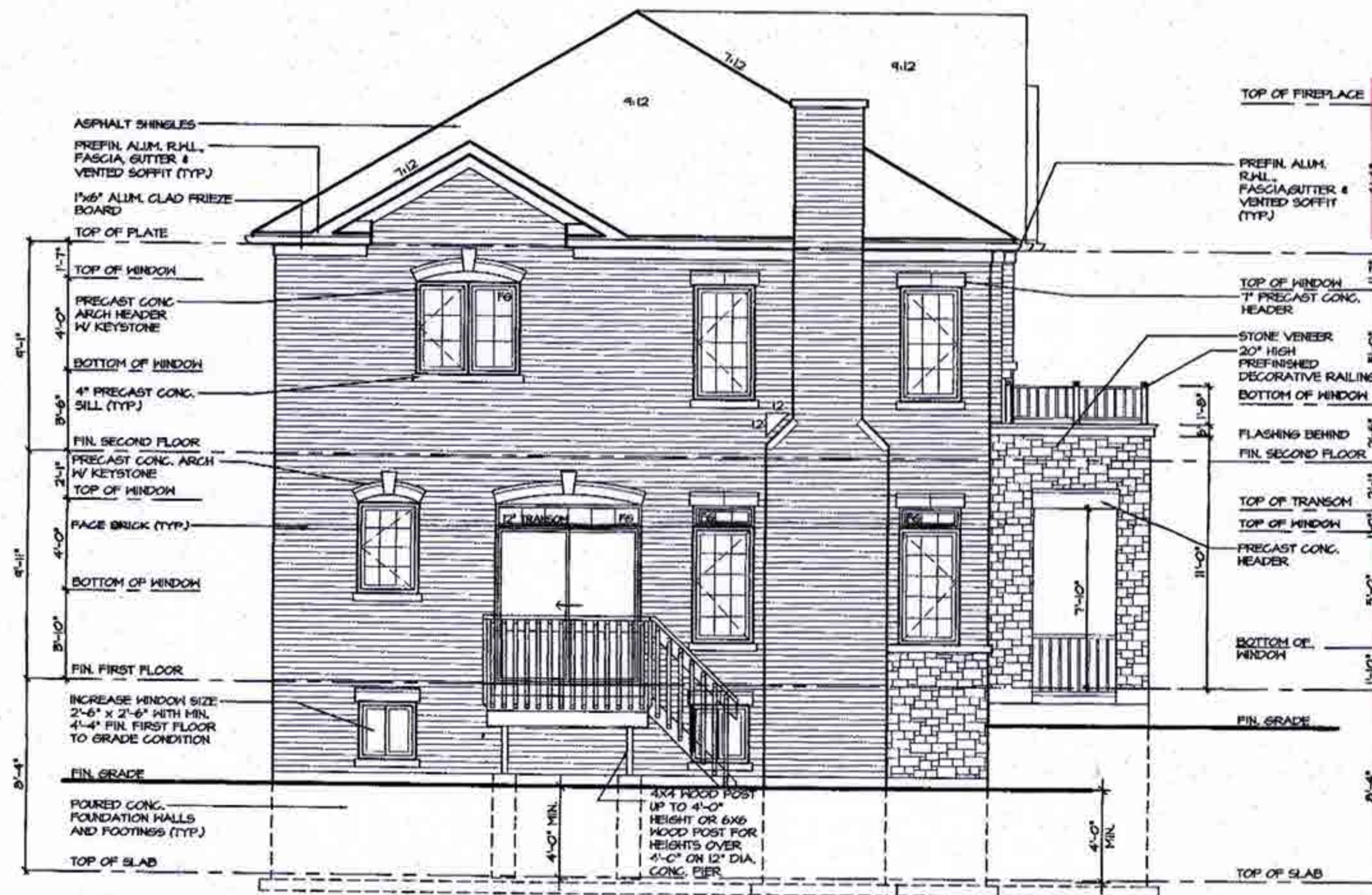
REAR ELEVATION 2 W.O.D. CONDITION
