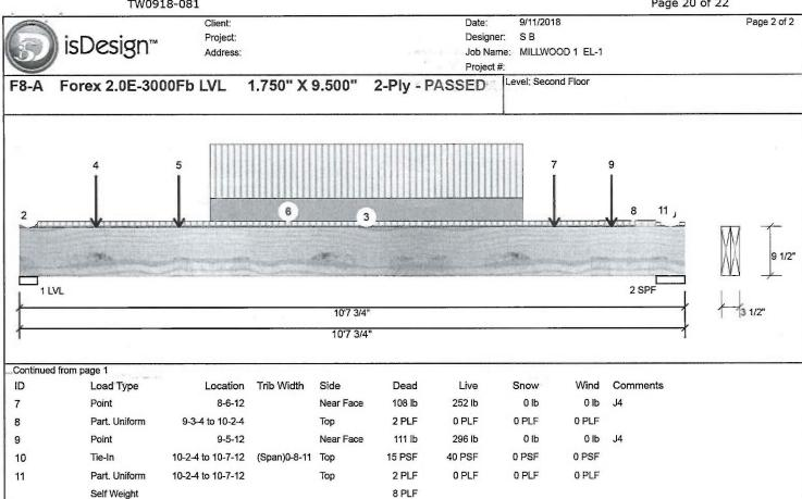
Pass-Thru Framing Squash Block is required at all point loads over bearings
