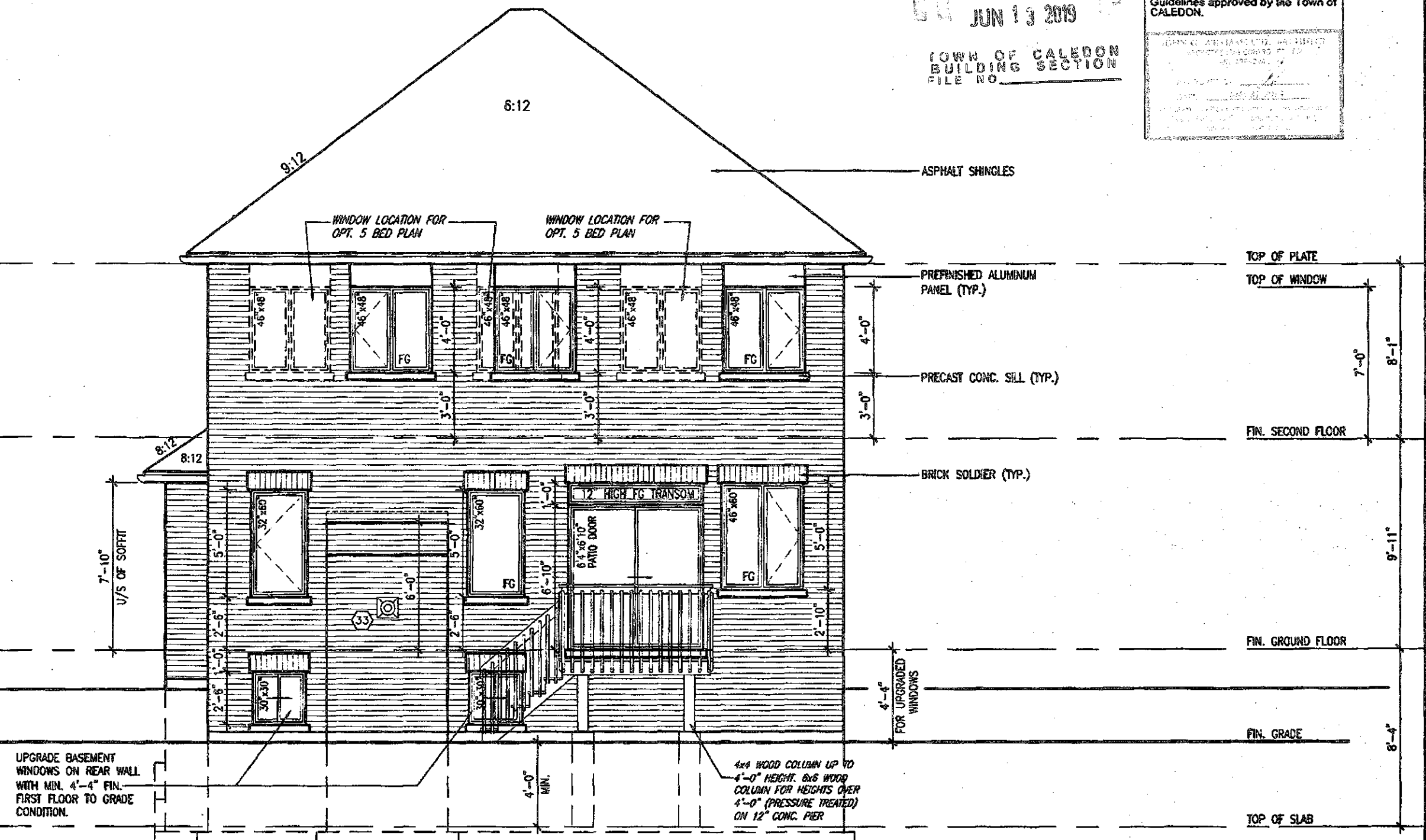
REAR ELEVATION 1'- DECK CONDITION
