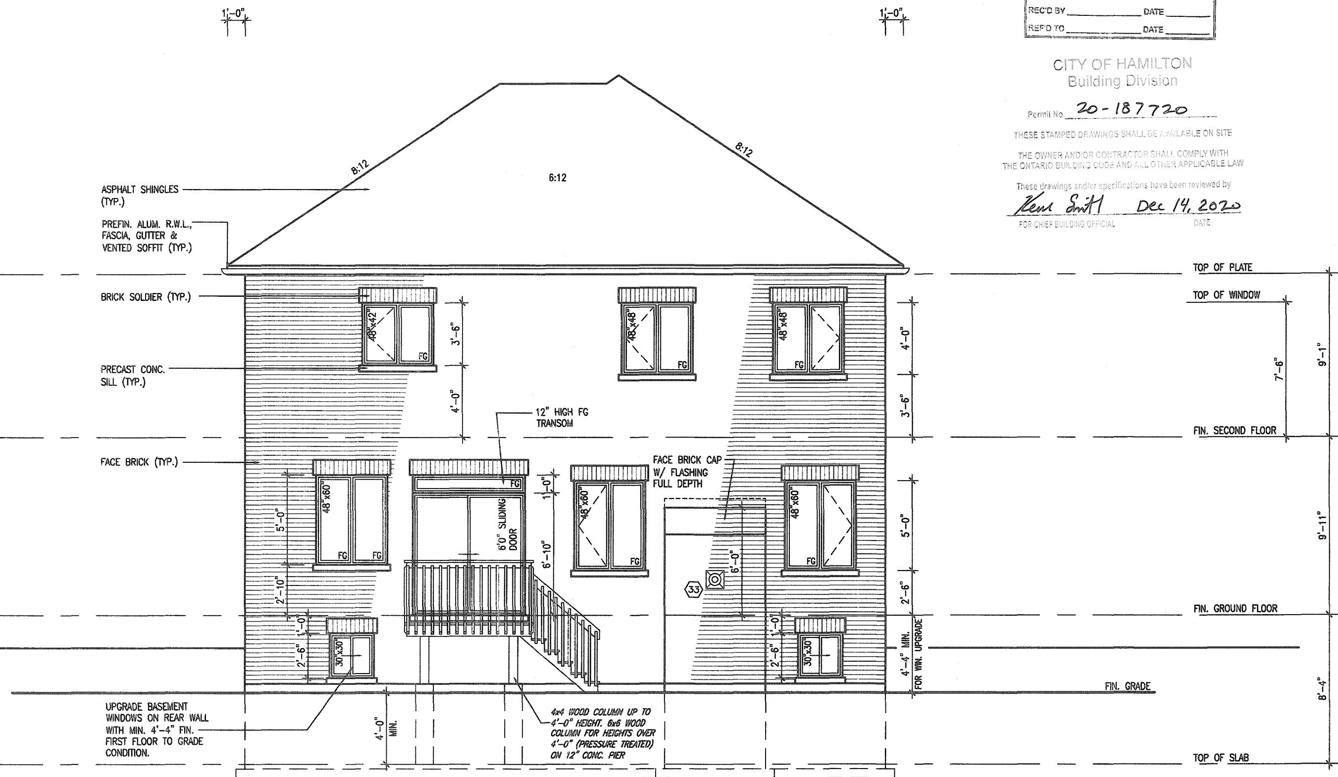
REAR ELEVATION '2'- DECK CONDITION DECK NOT REQUIRED
