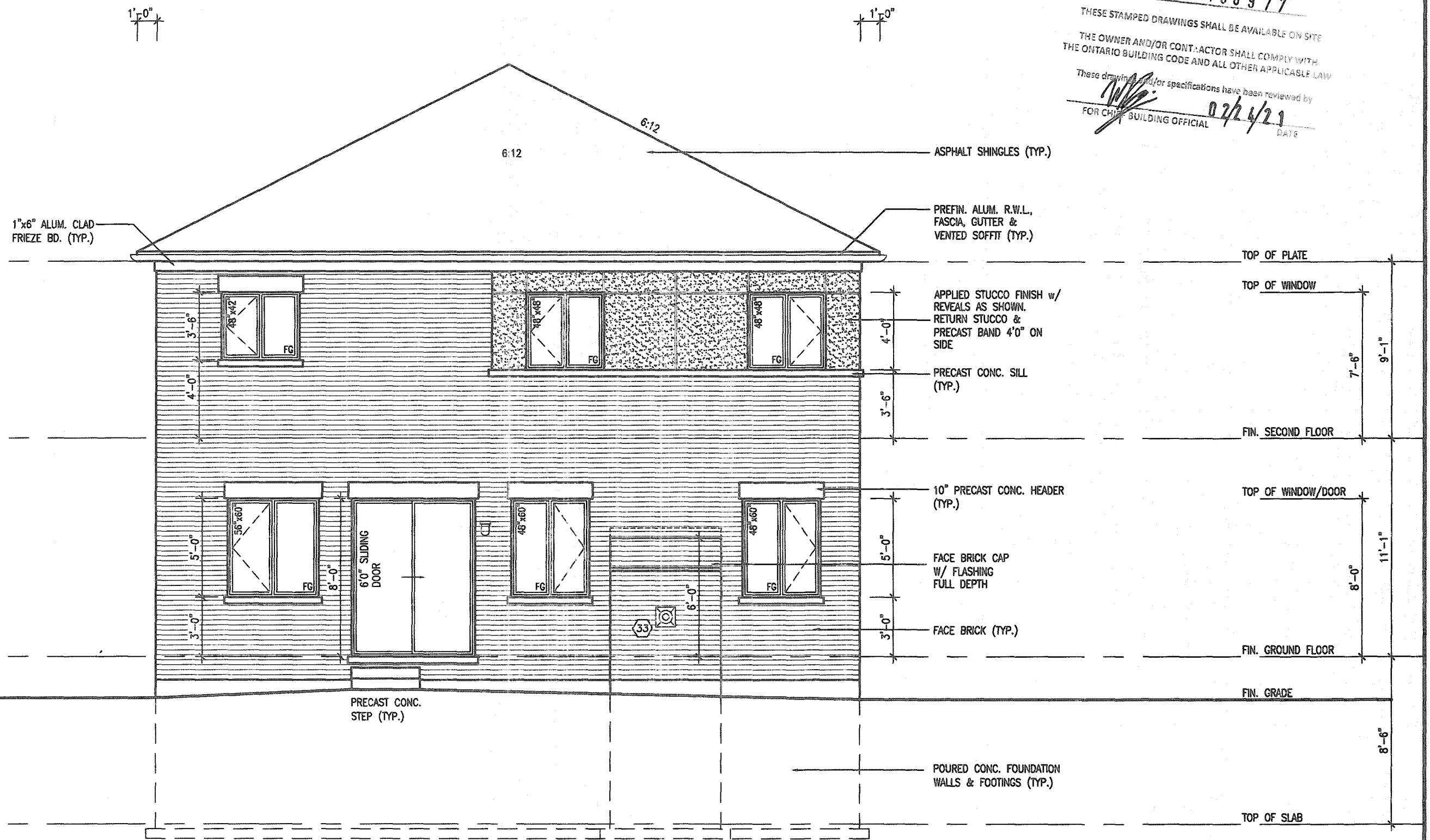
UPGRADED REAR ELEVATION - ELEV. '3'
