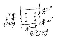
PROVIDE 3 ROWS OF 31/2" ARDOX SPIRAL NAILS @8 "O/C FOR MULTI-PLY NAILING, MAINTAIN A MIN. 2 LUMBER EDGE/END DISTANCE. DO NOT USE AIR KAILS
