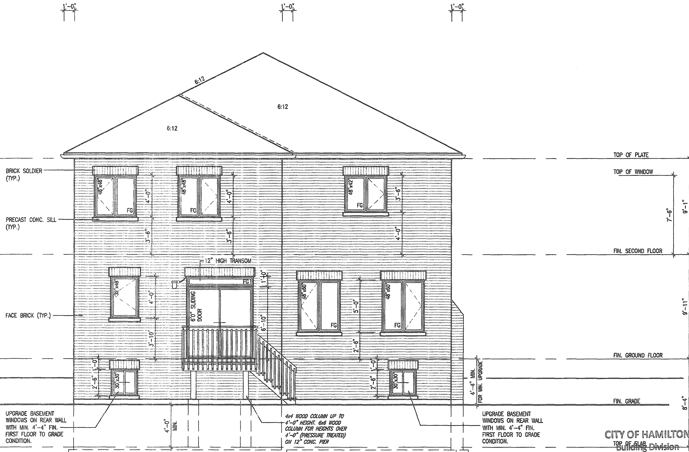
REAR ELEVATION '3'- DECK CONDITION
