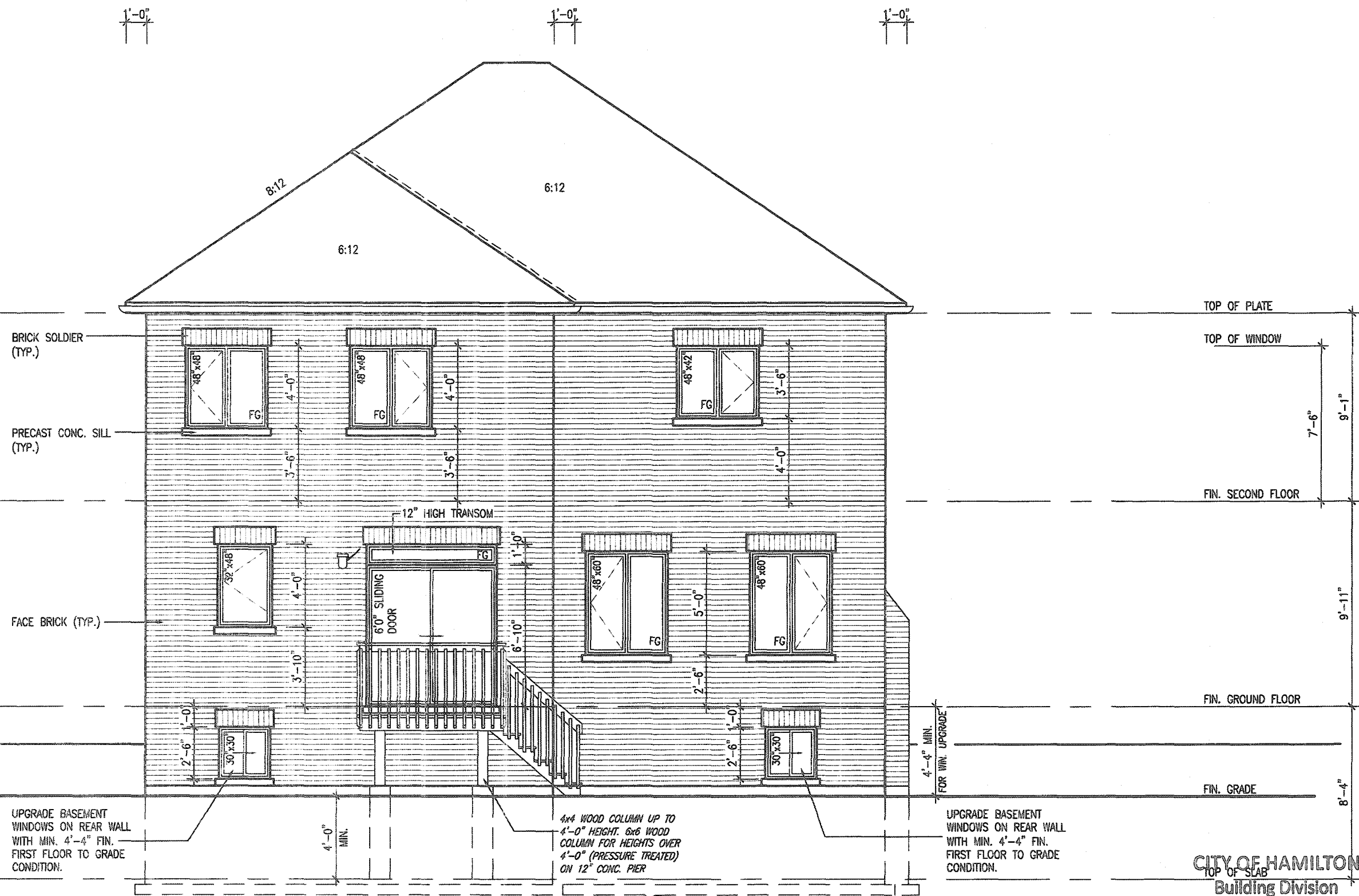
REAR ELEVATION '1'- DECK CONDITION
