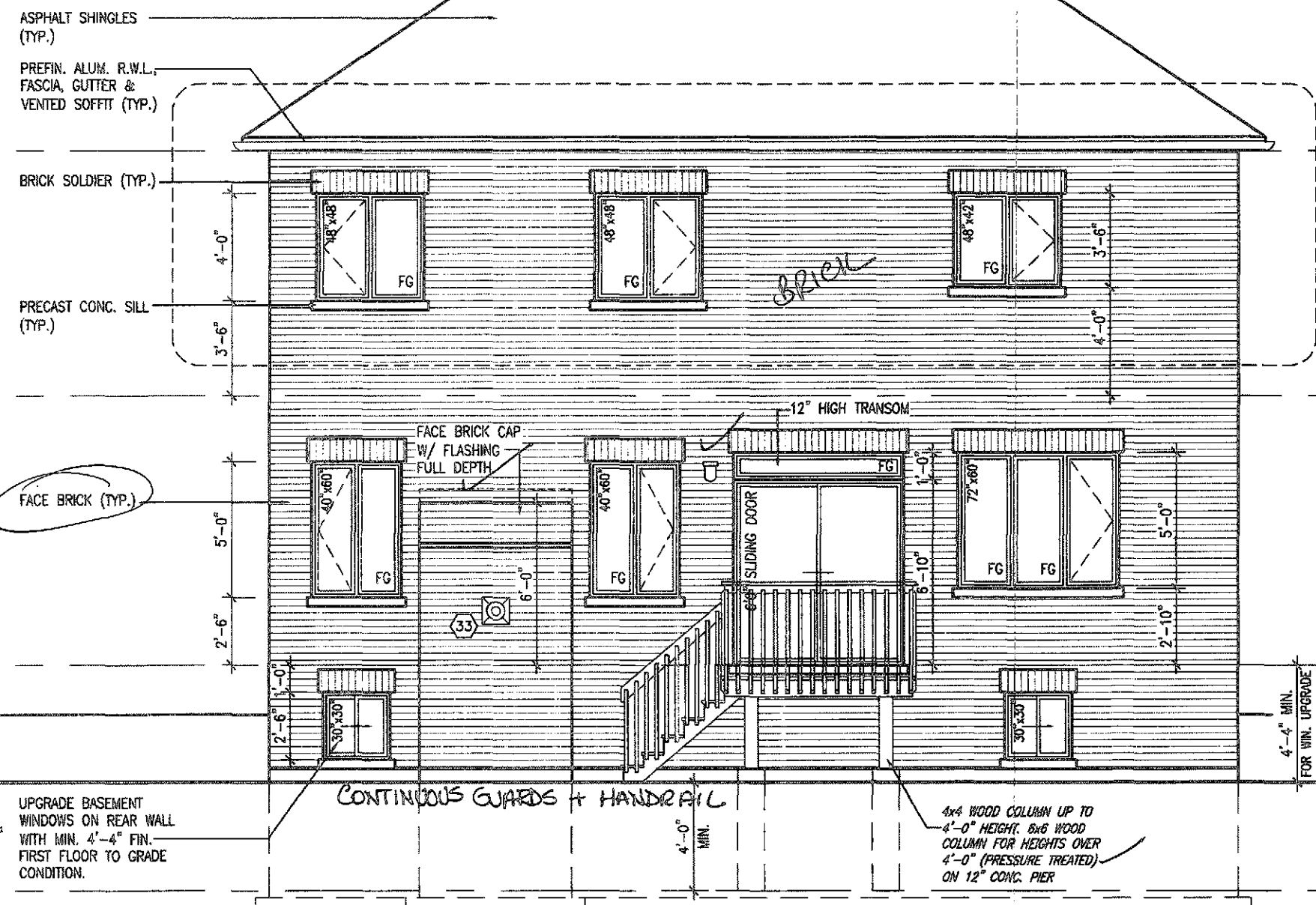
REAR ELEVATION '2'- DECK CONDITION
