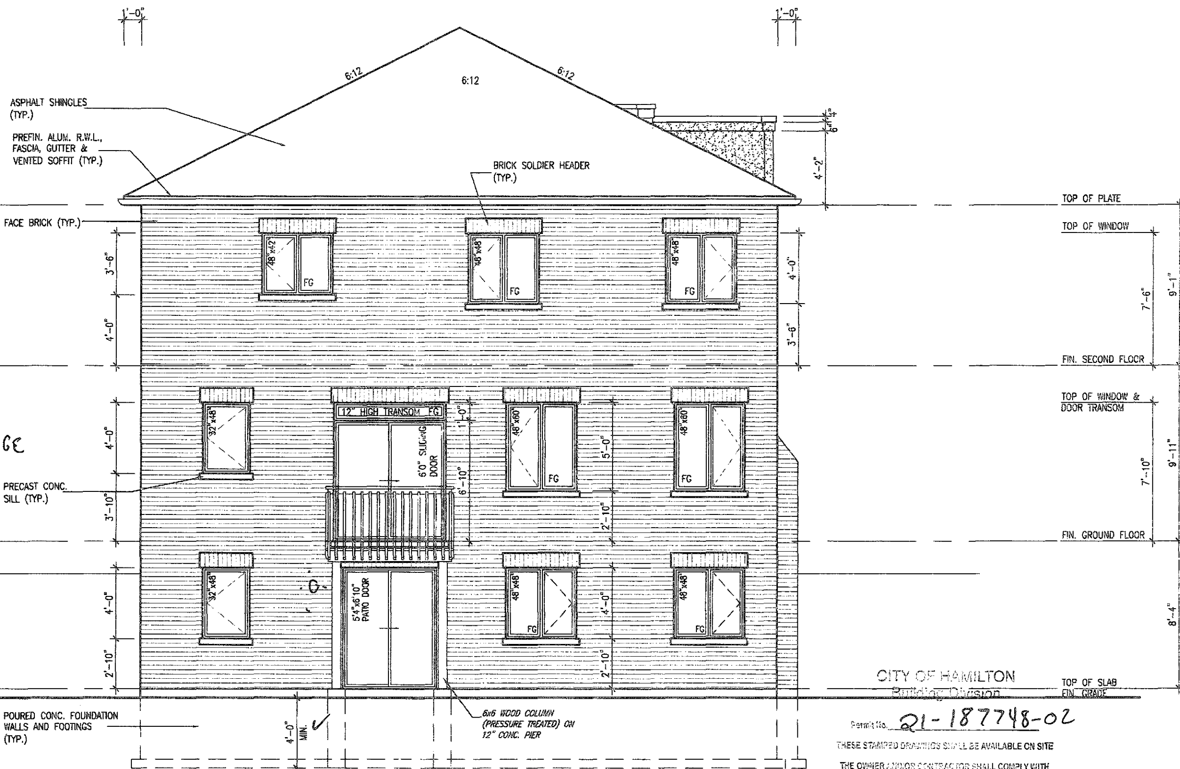
REAR ELEVATION '3' - WALK-OUT CONDITION
