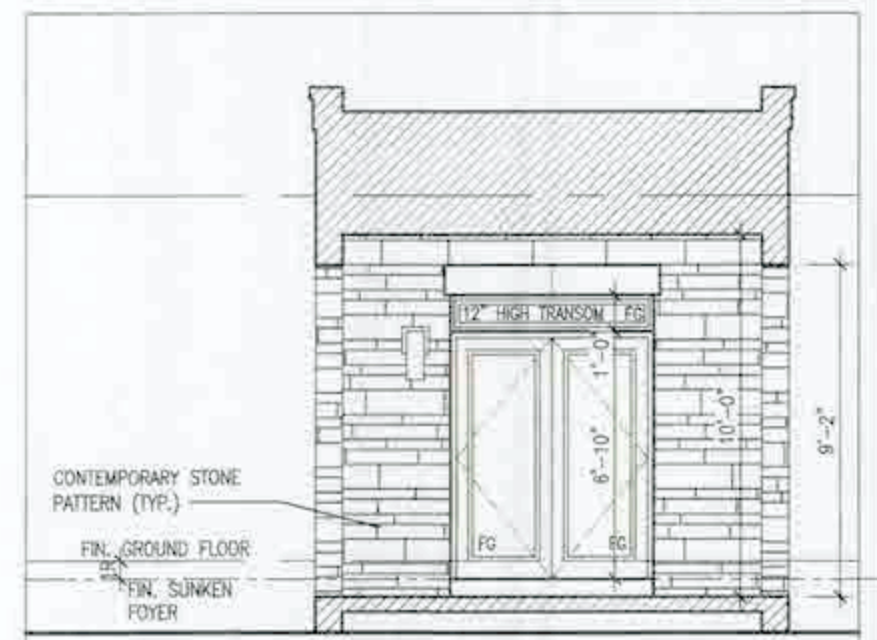
PORTICO INTERIOR ELEVATION '3'
