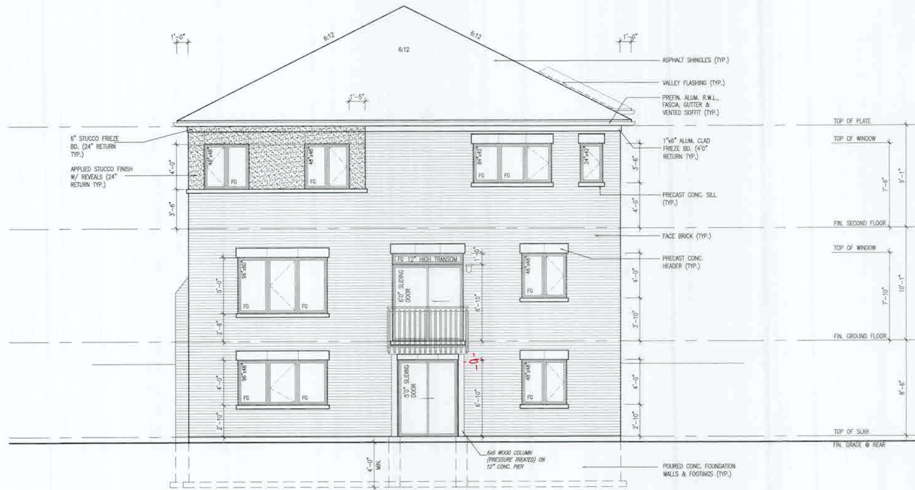
UPGRADED REAR ELEVATION - ELEV. '3' WALKOUT CONDITION
