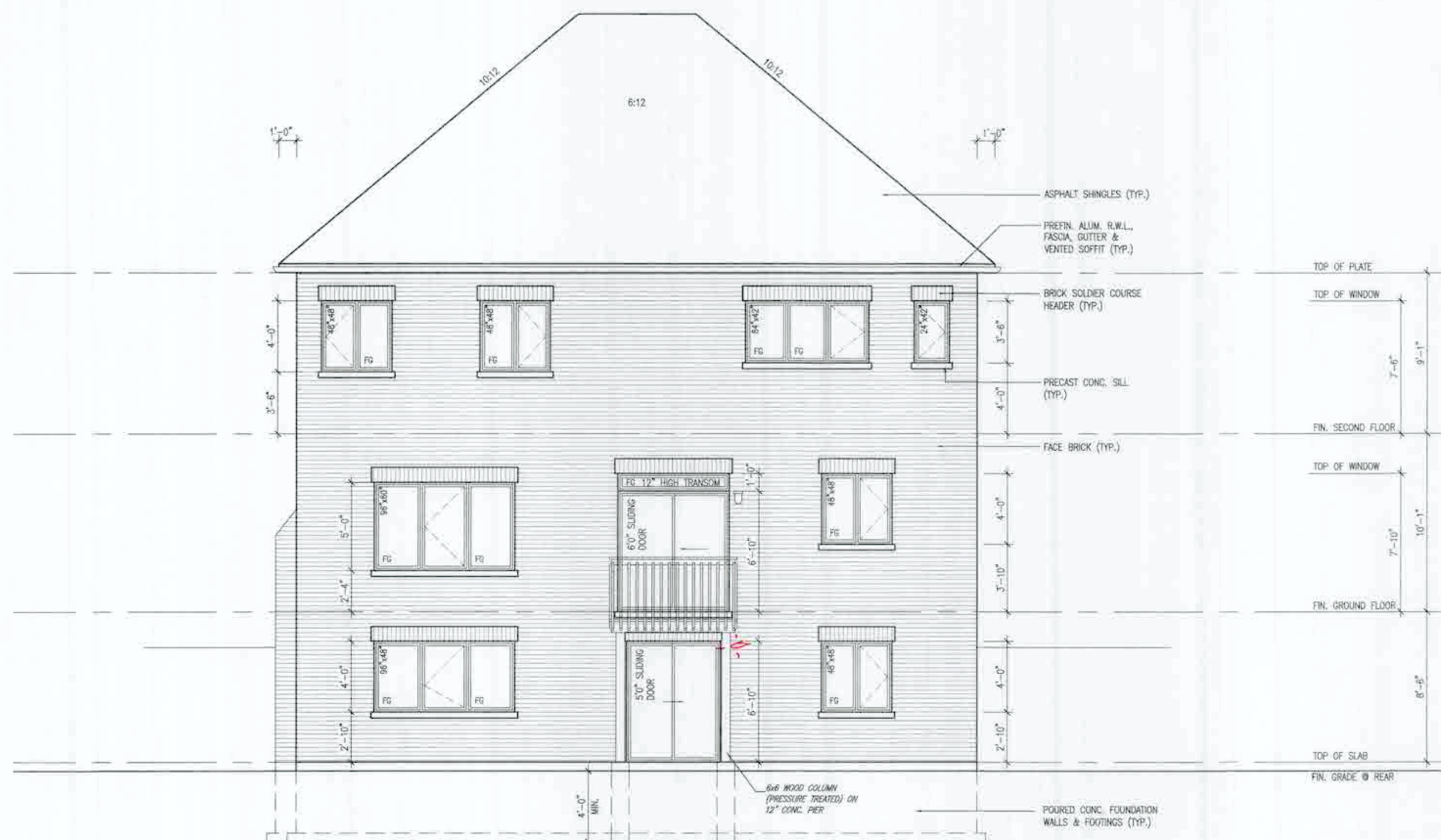
REAR ELEVATION - ELEV. '2' WALK-OUT CONDITION
