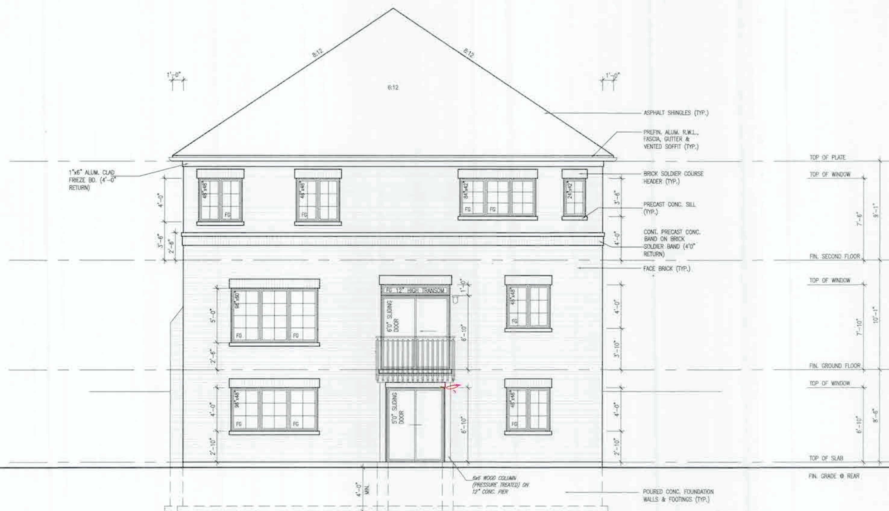
UPGRADED REAR ELEVATION - ELEV. '1' WALKOUT CONDITION
