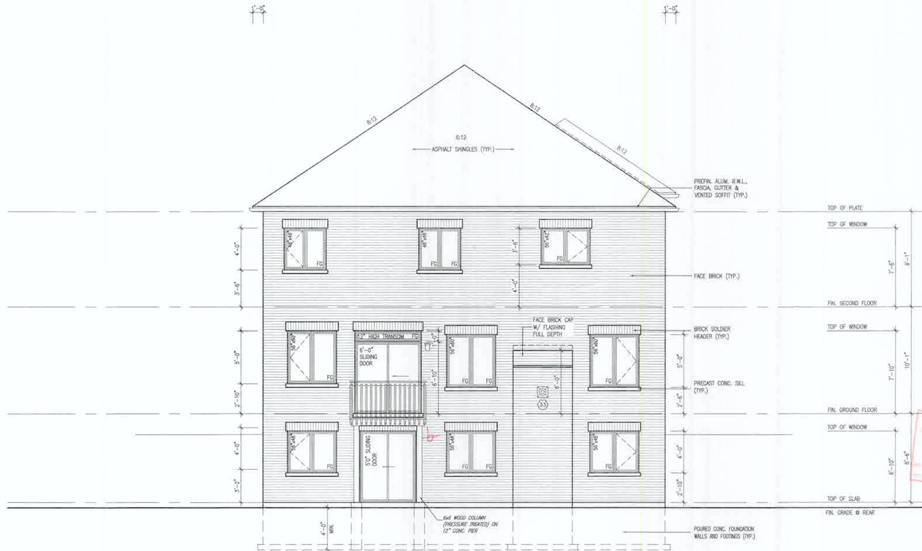
REAR ELEVATION '2' -WALK-OUT CONDITION
