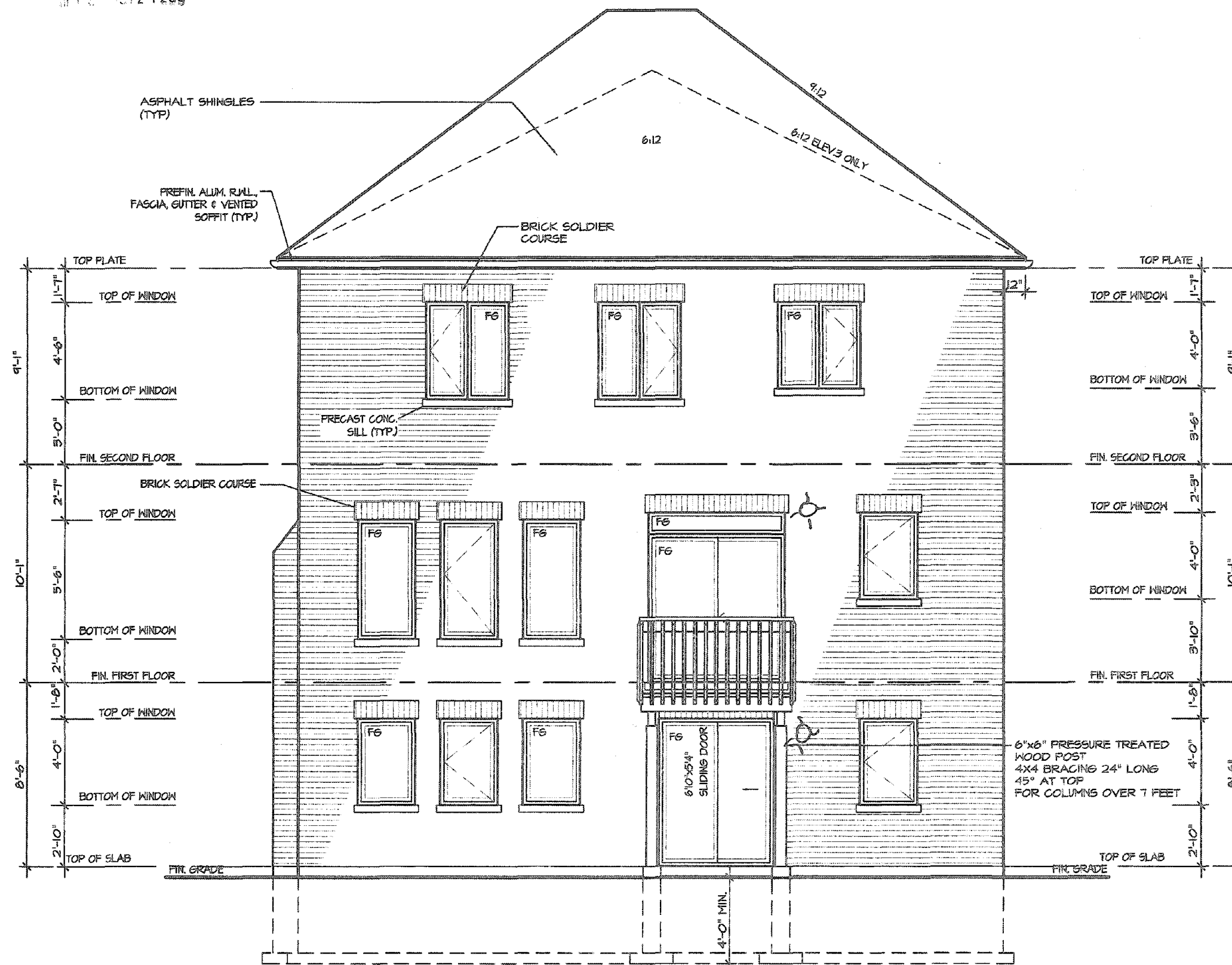
REAR ELEVATION 1, 2 & 3 WALKOUT CONDITION
