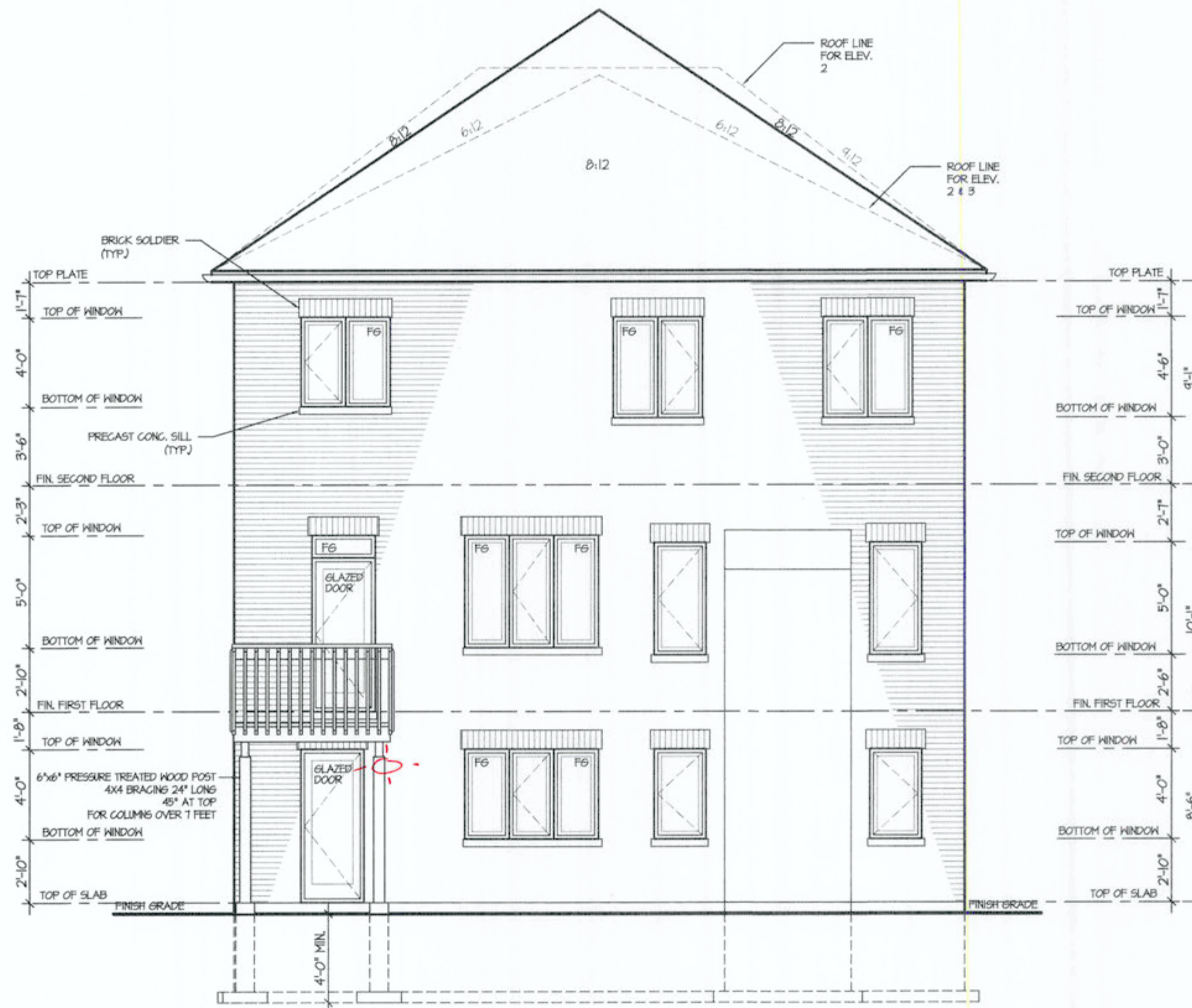
REAR ELEVATION 1, 2 & 3 WALKOUT CONDITION
