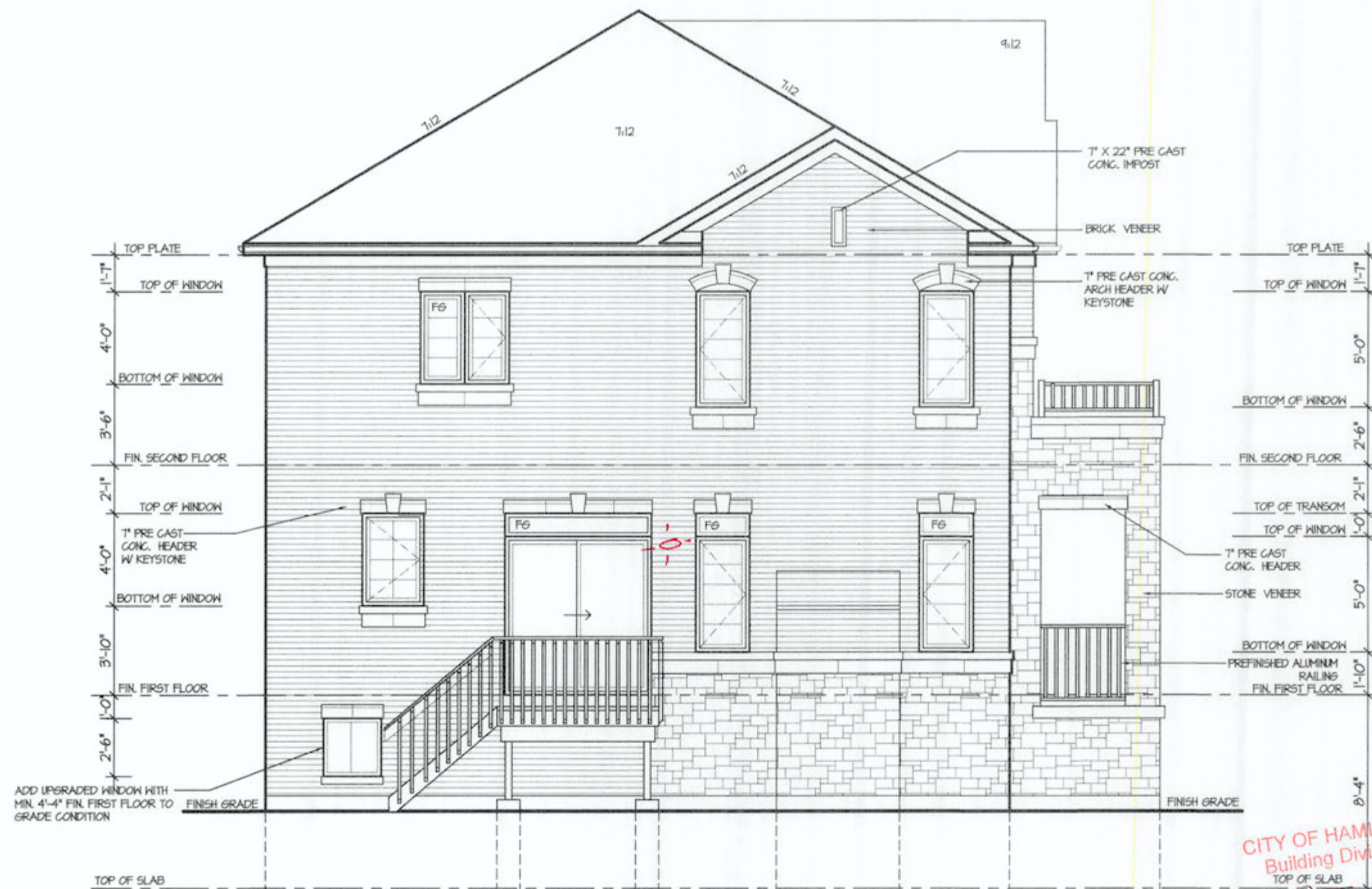
REAR ELEVATION 2 FOR DECK CONDITION
