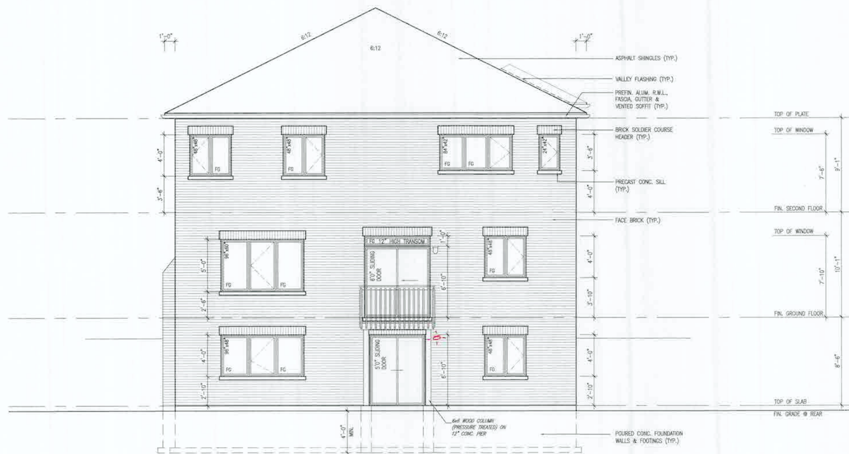
REAR ELEVATION - ELEV. '3' WALK-OUT CONDITION
