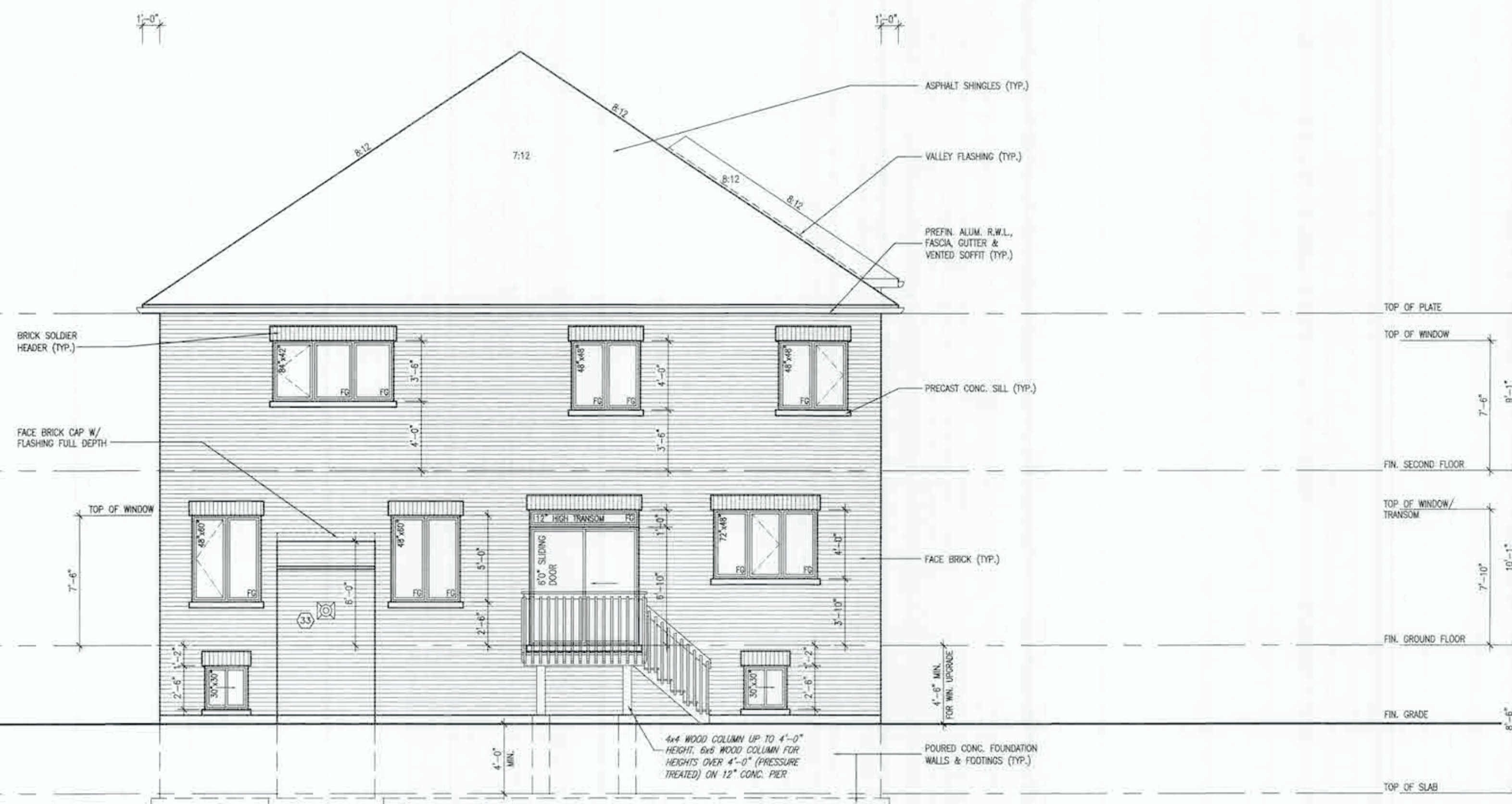
REAR ELEVATION - ELEV. '2' DECK CONDITION
