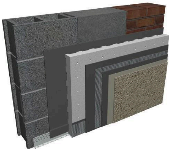
Figure 8. Puccs EIFS with moisture barrier over masonry, concrete, and brick
