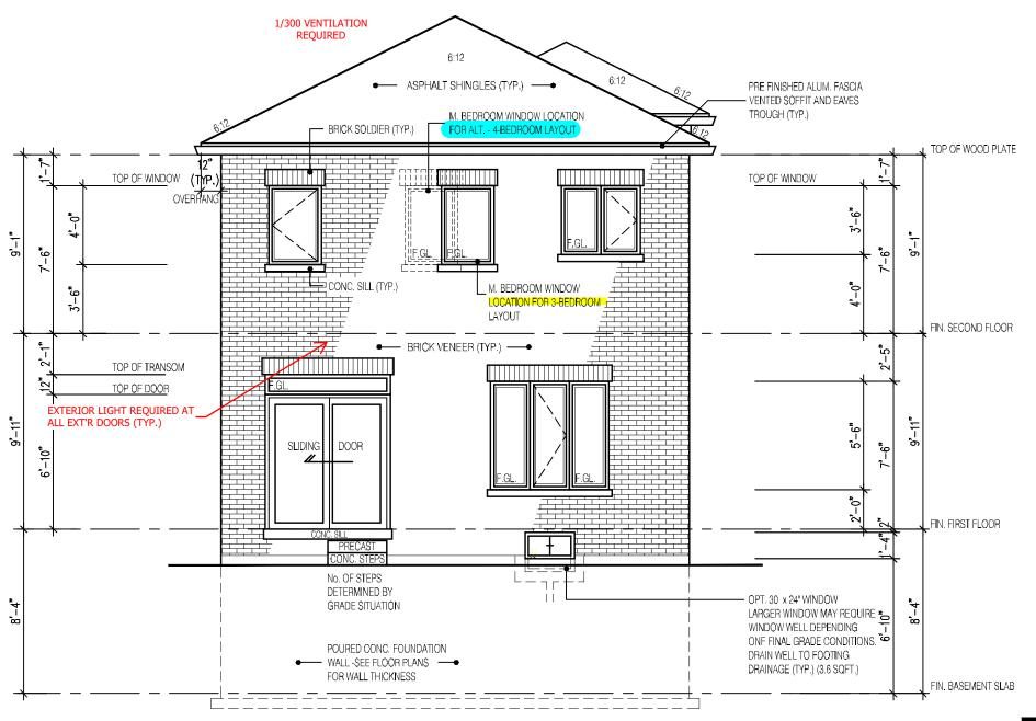
EXTERIOR CONCRETE STAIRS W/ MORE THAN 2 RISERS TO MEET THE REQUIREMENTS OF 9.8.9.2.(1)
