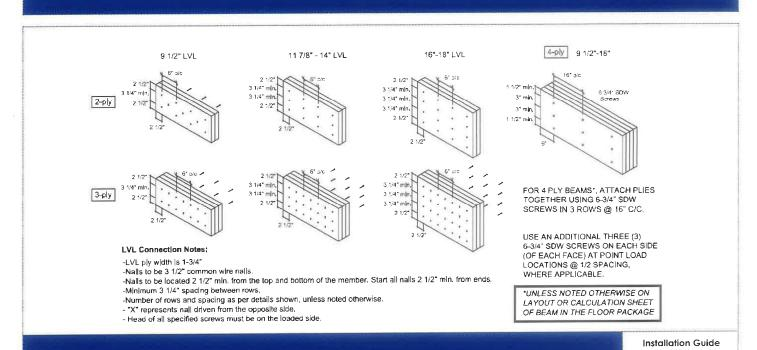
FOR MULTIPLE MEMBER CONNECTION OF BOISE ALLJOISTS REFER TO THE BOISE CASCADE INSTALLATION GUIDE
