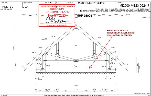
N. L. G. A. RULES CHORDS SIZE A - D 2x4 D - G 2x4 N - B 2x4 H - F 2x4 M - C 2x4 L - J 2x4 I - H 2x4 LUMBER No. 2 DESCR. SPF SPF SPF SPF SPF SPF SPF SPF SPF DRY DRY DRY DRY DRY DRY DRY DRY SPF ALL WEBS EXCEPT 2x3 DRY No.2 ALL GABLE WEBS 2x3 DRY DRY: SEASONED LUMBER. No.2 GABLE STUDS SPACED AT 2-0-0 OC.
