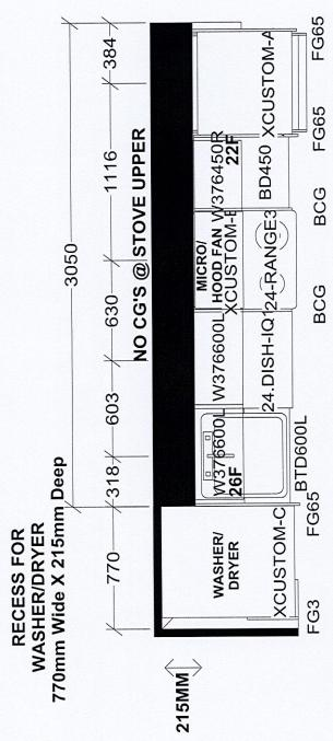
ASSEMBLE CABINET FOR WASHER/ DRYER ON SITE
