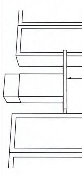
\*The supplied duct cover fits 7'-7" to 10'-6" ceiling heights (12' ceiling height with optional high celling kit UX12DC9SLSS/UX12DCBLTS) (14' ceiling height with optional high celling kit UX14DC9SLSS/UX14DC9BLTS)
