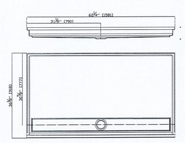
HANDICAP ACCESSIBLE LINEAR DRAIN PREVENTS WATER RUN-OFF TO FLOOR
