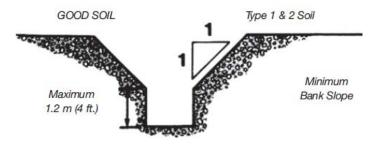
**3.5.2** Type 3 soil: Cut walls back at an angle of 1-to-1, but from the bottom of the trench.
