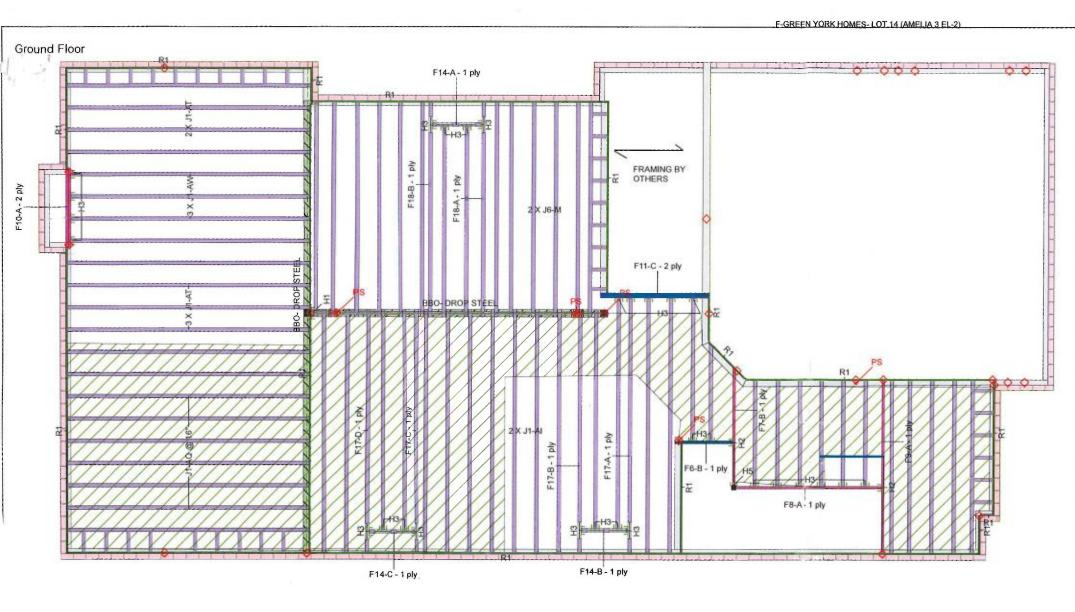
1. The loads used in the calculation of the attached approved components conform to the floor assembly shown on this layout.
