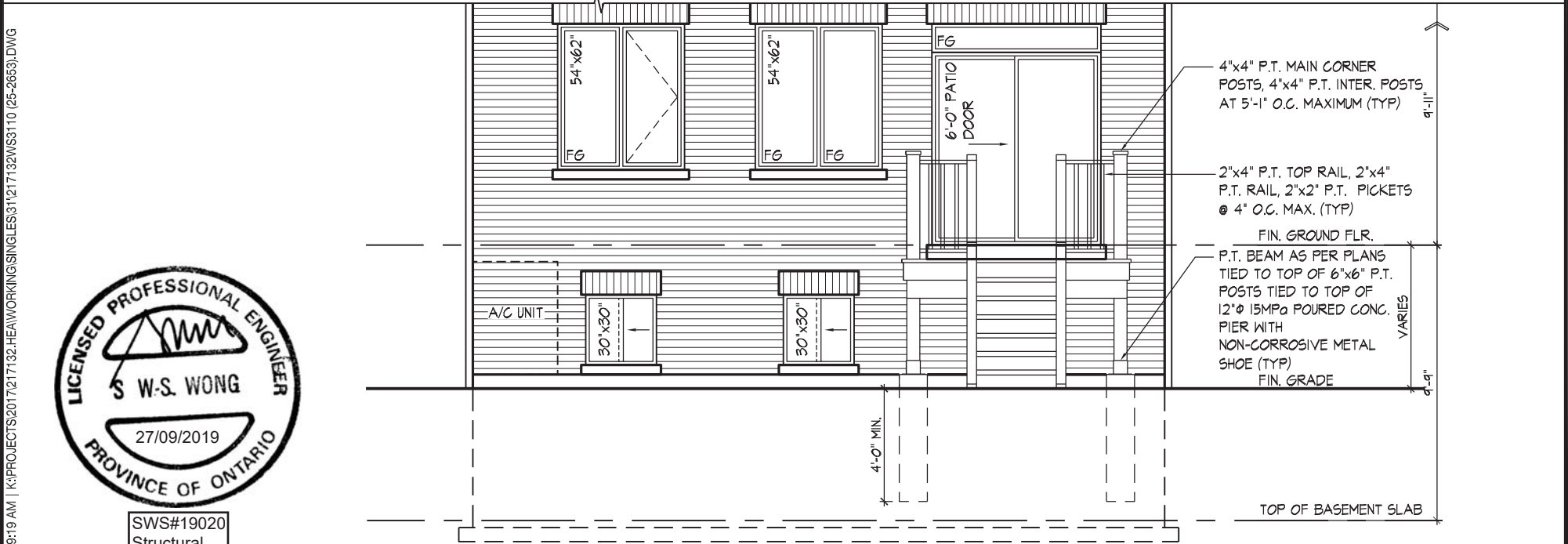
PART REAR ELEVATION 'A' - L.O.D. CONDITION (ELEV. 'B','C' & 'D' SIMILAR)
