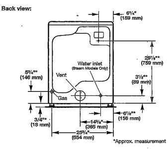
NOTE: Most installations require a minimum of 5" (127 mm) clearance behind dryer for exhaust vent with elbow. See "Venting Requirements."
