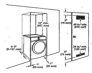
0" (0 mm) rear spacing is allowed for straight back venting only. For steam models only, inlet hose must not be kinked.
