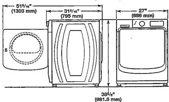
All dimensions show minimum spacing allowed. For each arrangement, consider allowing more space for ease of installation and servicing, and spacing for companion appliances and clearances for walls, doors, and floor moldings.
