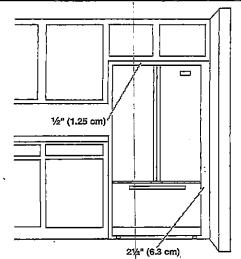
To ensure proper ventilation for your refrigerator, allow for a ½" (1.25 cm) space on each side and at the top. Allow for 1" (2.54 cm) of space behind the refrigerator. If your refrigerator has an ice maker, make sure you leave some extra space at the back for the water line connections.
