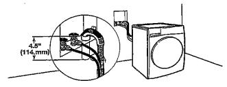
See requirements for floor standpipe drain system.
