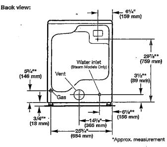
NOTE: Most installations require a minimum of 5" (127 mm) clearance behind dryer for exhaust vent with elbow. See "Venting Requirements."
