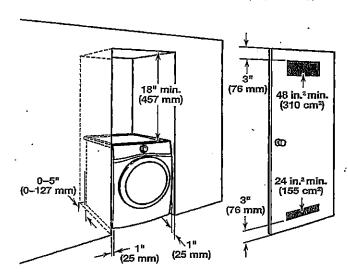
0" (0 mm) rear spacing is allowed for straight back venting only. For steam models only, inlet hose must not be kinked.
