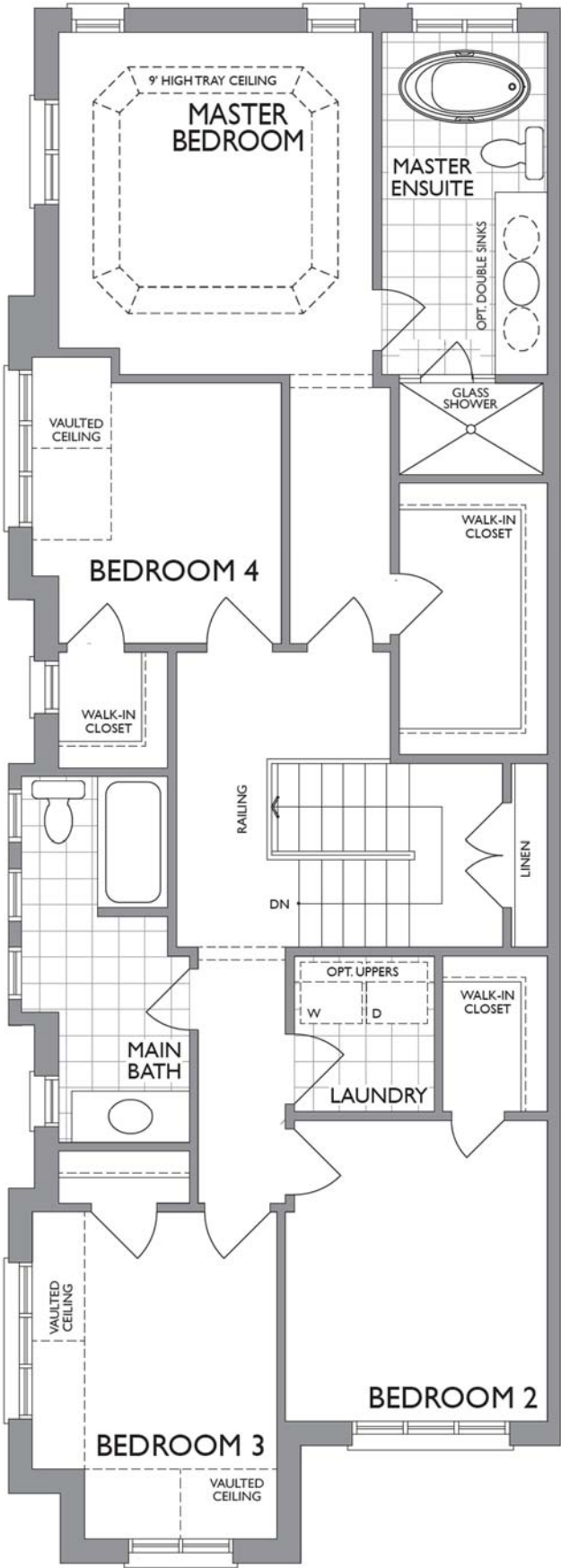
ALT. SECOND FLOOR - 4 BEDROOMS ELEVATION B
