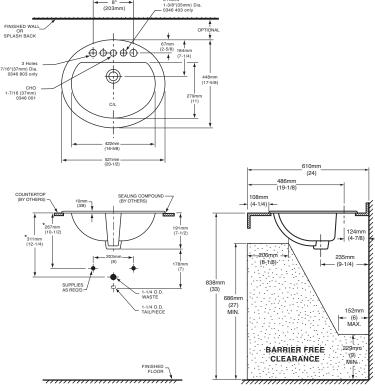
\* DIMENSIONS SHOWN FOR LOCATION OF SUPPLIES AND "P" TRAP ARE SUGGESTED. FOR COUNTERTOP CUTOUT AND INSTALLATION INSTRUCTIONS USE TEMPLATE SUPPLIED WITH SINK.
