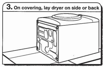
Place a covering, such as cardboard or a blanket, on the floor to avoid damage. Gently lay the dryer down with its side or back on the covering.
