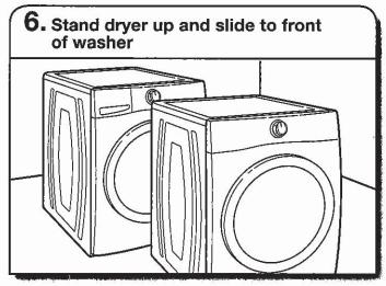
Lift the dryer back to an upright position, keeping it on the cardboard (or carton bottom). Use the cardboard to slide the dryer to the front of the washer to avoid damaging the rubber feet.
