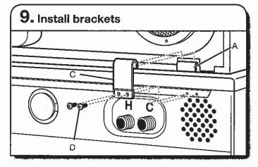
Push the hooked end of the bracket (C) down over the plastic clip (A). A flat-blade screwdriver may help to seat the bracket over the plastic clip. Slide the dryer forward as needed and attach bracket (C) to washer with pan-head screws (D). Tighten screws securely. Repeat on other side.
