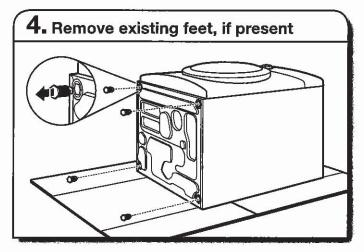
Using a wrench or slip-joint pliers, remove the existing feet if present.
