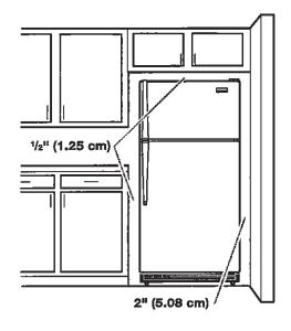
To ensure proper ventilation for your refrigerator, allow for a %" (1.25 cm) space on each and between overhead cabinets and refrigerator top. Allow at least 1" (2.5 cm) between back of cabinet and the wall. If your refrigerator has an ice maker, make sure you leave some extra space at the back for the water line connections.
