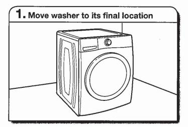
Leave room to work behind washer. Do not remove the shipping bolts.
