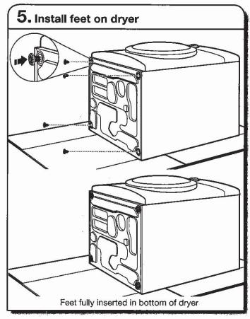
Using a wrench or slip-joint pliers, install the new feet, turning them fully into the bottom of the dryer.
