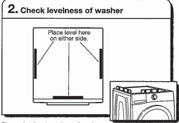
Place a level on top edges of washer, checking each side and front. If not level, tip washer and adjust feet up or down as shown in Installation Instructions, repeating as necessary.
