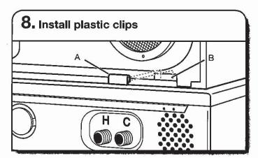
Remove the plastic clips (2), brackets (2), and pan-head screws (4) from the parts bag. Take a plastic clip (A) and, with the flat side facing out, push it down onto the lower edge of the slot (B) in the dryer back. A flat-blade screwdriver may help to open the plastic clip slightly. Repeat on other side.
