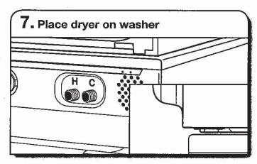
Lift the dryer up and set securely on top of washer. Position dryer to slightly overhang the back of the washer – too much overhang will allow the rear feet to slip off the back of the washer top.
