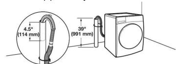
Minimum diameter for a standpipe drain: 2" (51 mm). Minimum carry-away capacity: 17 gallons (64 L) per minute. A 1/4" (6 mm) diameter to 1" (25 mm) diameter Standpipe Adapter Kit is available; refer to the Quick Start Guide for online ordering information. Top of standpipe must be at least 39" (762 mm) high; install no higher than 96" (2.4 m) from bottom of washer. If you have an overhead sewer and need to pump higher than 96 (2.4 m), a sump pump and associated hardware are needed. See
