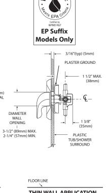
2 1/2" MAX. (63mm) 6'-6" (1981mm) NOMINAL 4-1/2" (114mm) WALL OPENING SHOWER 48" (1219mm) 32" (813mm) (133mm AND TUB ONLY **THICK WALL APPLICATION THIN WALL APPLICATION CRITICAL DIMENSIONS**
