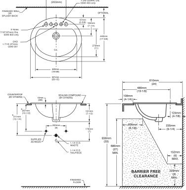
\* DIMENSIONS SHOWN FOR LOCATION OF SUPPLIES AND "P" TRAP ARE SUGGESTED. FOR COUNTERTOP CUTOUT AND INSTALLATION INSTRUCTIONS USE TEMPLATE SUPPLIED WITH SINK.
