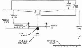
NOTES: \*DIMENSIONS SHOWN FOR LOCATION OF SUPPLIES AND "P" TRAP ARE SUGGESTED. FAUCETS NOT INCLUDED WITH FIXTURE AND MUST BE ORDERED SEPARATELY. FOR COUNTERTOP CUTOUT AND INSTALLATION INSTRUCTIONS USE TEMPLATE SUPPLIED WITH SINK.
