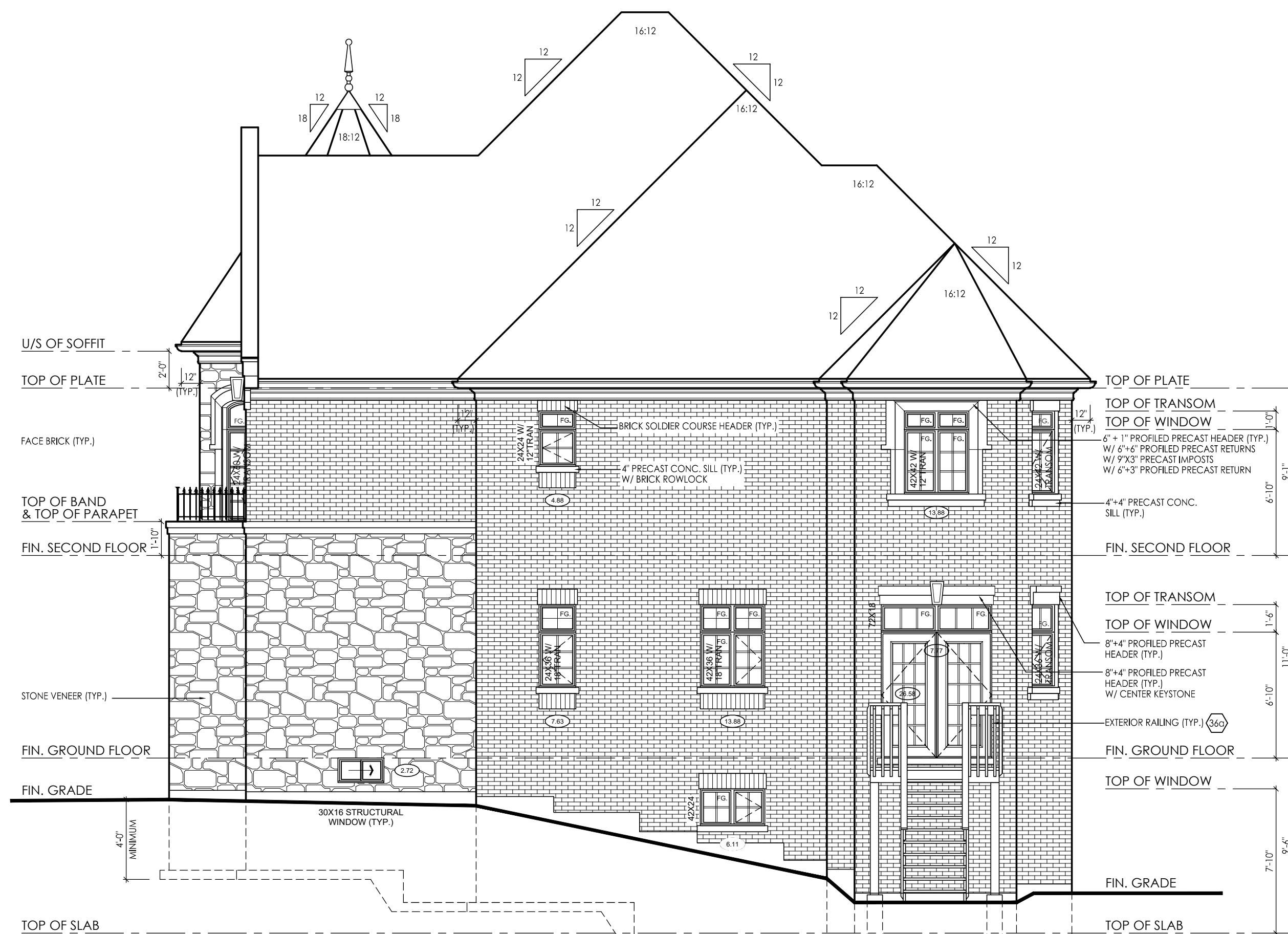
RIGHT SIDE ELEVATION 'A' LOB CONDITION - LOT 39
