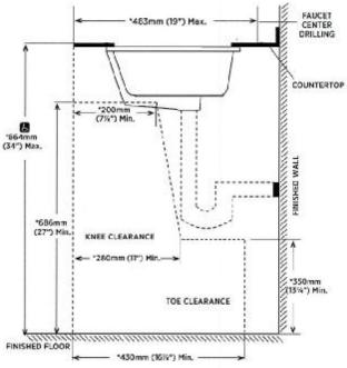
IOTE: \* Starred measurements comply with CSA B6SI and OBC barrier free accessibility requirements.
