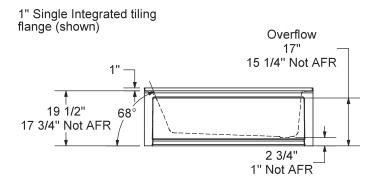
Wood support design may vary. Single Integrated tiling flange: 1" height x 1/4" thickness (shown)
