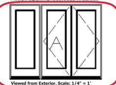
V Double Door Mull (NoShp) (OA Frame= 99 1/16 x 81 5/8 ) Factory Mull Int= , \*\*(Ext= Smoke)\*\* , ,Jamb= 6 5/8 , ,BOX= NO MODEL ,MODEL= NO MODEL ,REINFORCEMENT= NO
