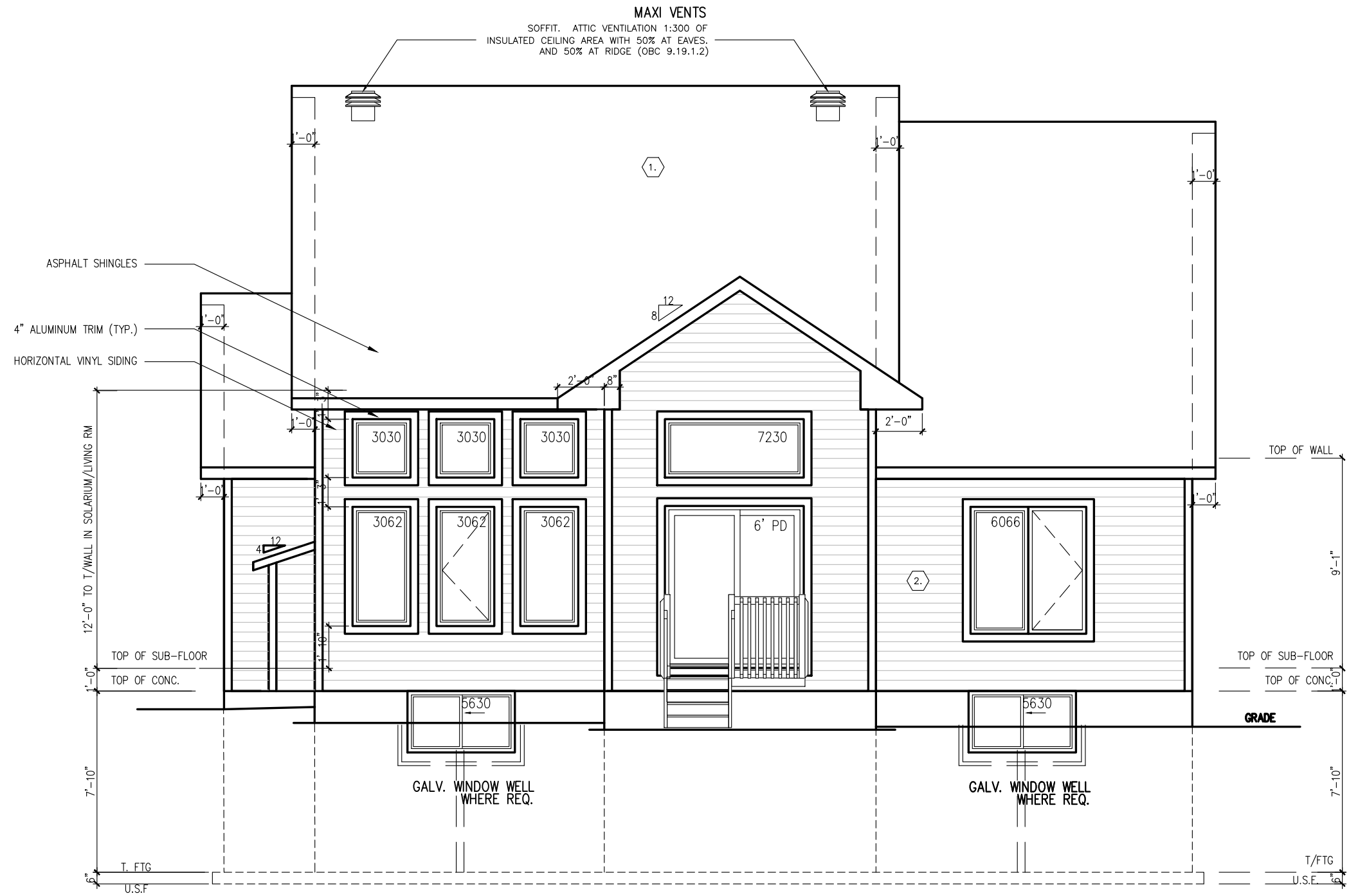
ELEVATION C SUN ROOM REAR ELEVATION
